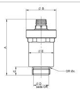
Installation The valve has to be positioned on the highest point of the plant and exclusively in vertical position. The valve operates automatically when the cap is unscrewed by 2 or 3 turns.
